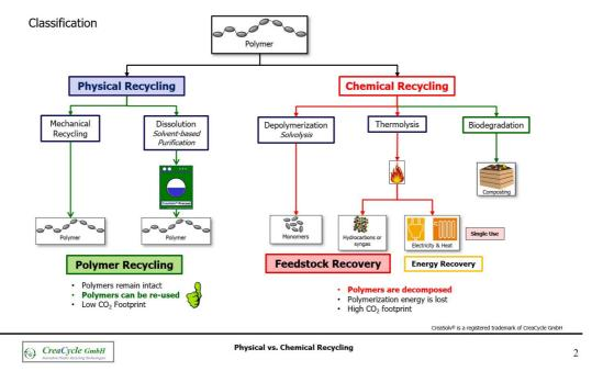
When mechanical recycling needs a high sorting purity of waste streams and fails on imbedded hazardous impurities or multilayer packaging, the CreaSolv<sup>®</sup> Process works like a washing machine on a molecular level.
