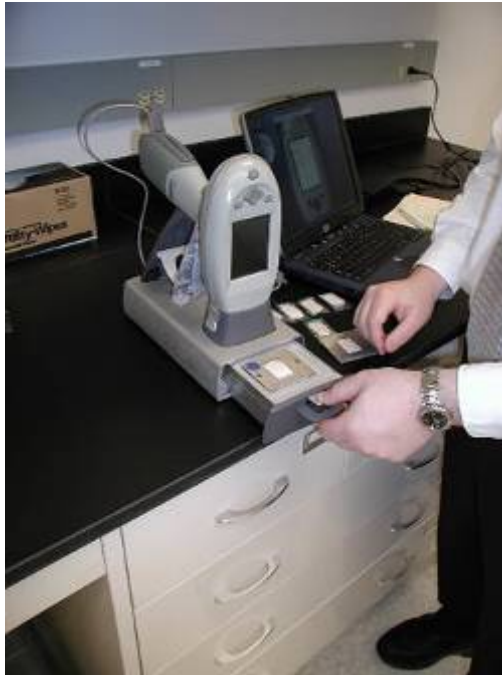
The Niton XLt incorporates a hand-held X-ray tube
