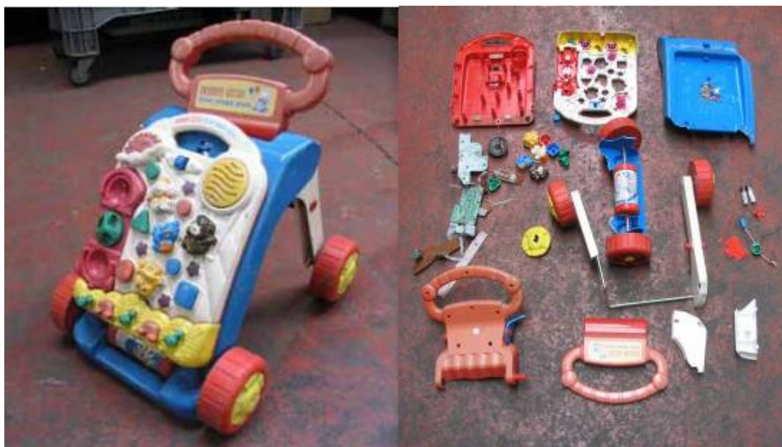
Child's electronic toy before and after dismantling into components and polymer types
