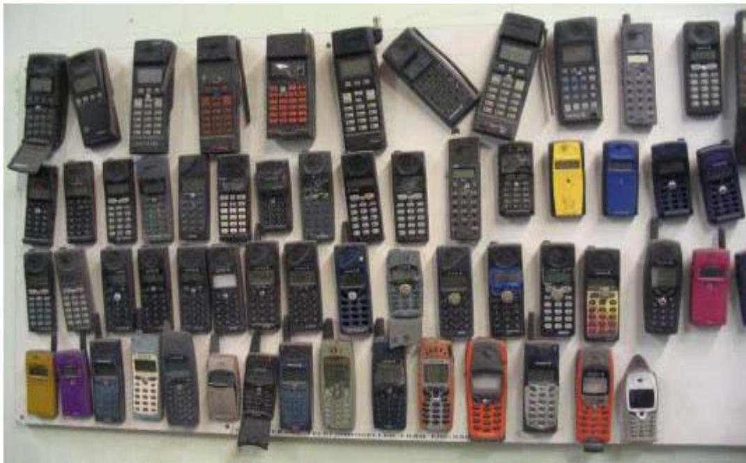
Mobile phones: an example where dismantling effort and cost is high and polymer recovery is low
