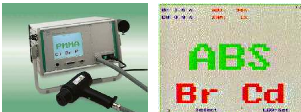
The SlideSpec-S2 sliding spark spectrometer (left) and typical screen display (right)
